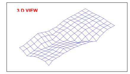
You can now view the complete ground profile in three Dimension from any angle. This 3D View helps in better interpretation of the ground area and for easy data checking.
