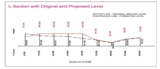
Program generates the sections in both X & Y directions as shown. It has an in-built Grid list from which you can select any number of sections. You can control all the drawing parameters such as section arrangement, ordinates and text size.
