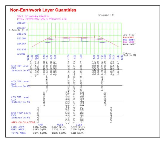
Following levels are entered at each chainage, on both Left and Right sides :
